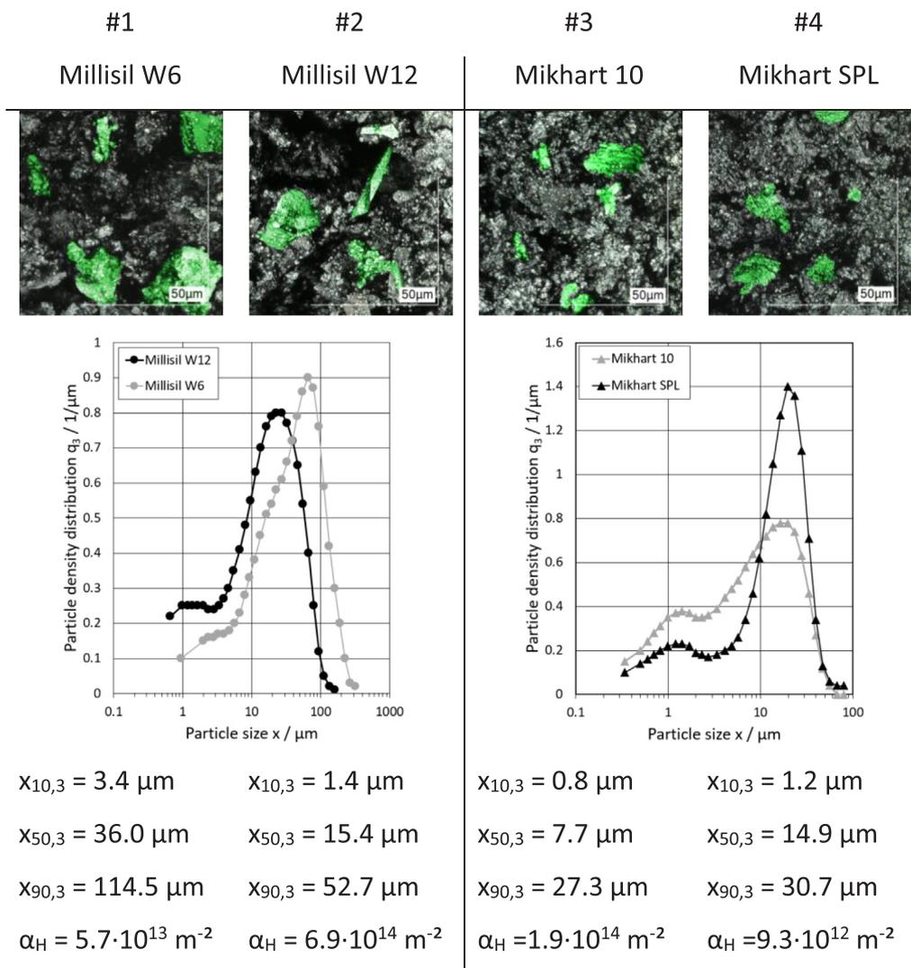
Fig. 4. Particle systems Investigated for cake discharge in the gas phase. The shape of the particles is orthorhombic. The particle sizes results in high specific flow resistances  $\alpha_H$  (VDI 2762-2).
