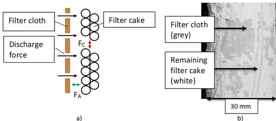
Fig. 1. Force condition inside a filter cake during the backwash procedure (a). Adhesion ( $F_A$ ) has to be smaller than the discharge force. If these conditions are not fulfilled, particles remain on the filter surface (b).
