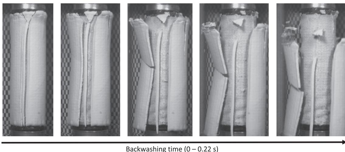
Fig. 5. Regeneration of the lab-scale candle filter (Millisil W6;  $H_{FC} = 1.5$  mm;  $\Delta p_{\text{Backwash}} = 1$  bar). Discharge in the liquid phase under the same conditions takes six times longer.
