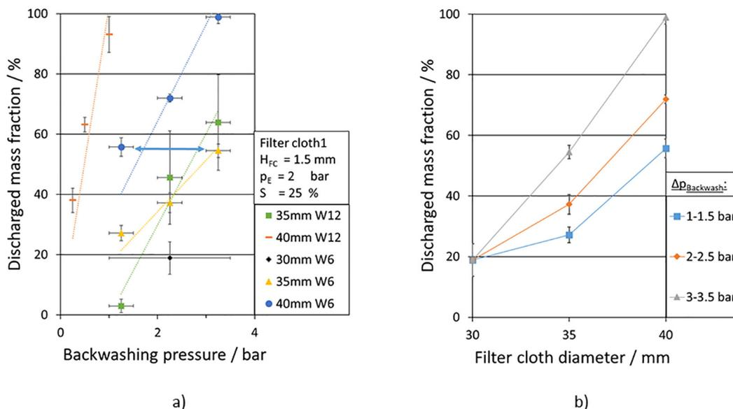
Fig. 6. Discharged mass fraction of the lab-scale candle filter as a function of the backwashing pressure (a) and the diameter of the filter cloth 1 (b) at a constant filter cake thickness  $H_{FC} = 1.5$  mm.
