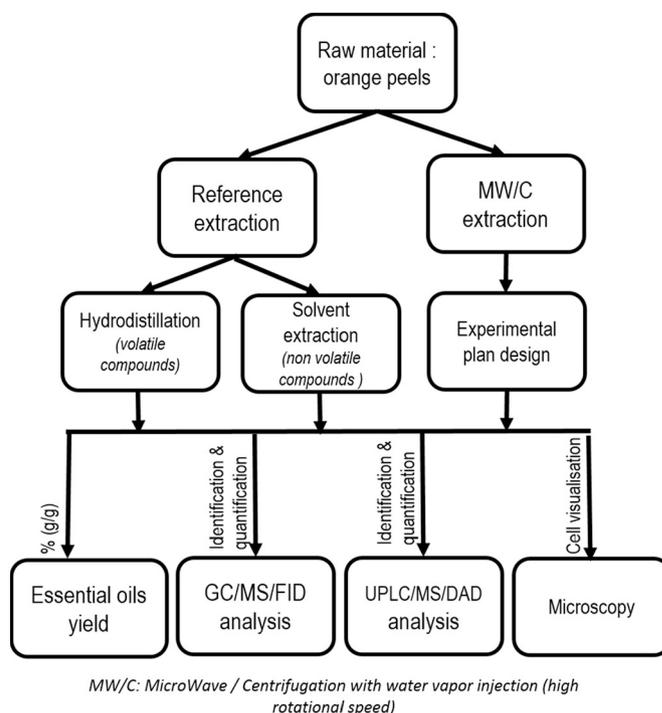
Fig. 1. Protocol treatment of orange peels by microwave and centrifugal force (MW/C) and reference extractions.
