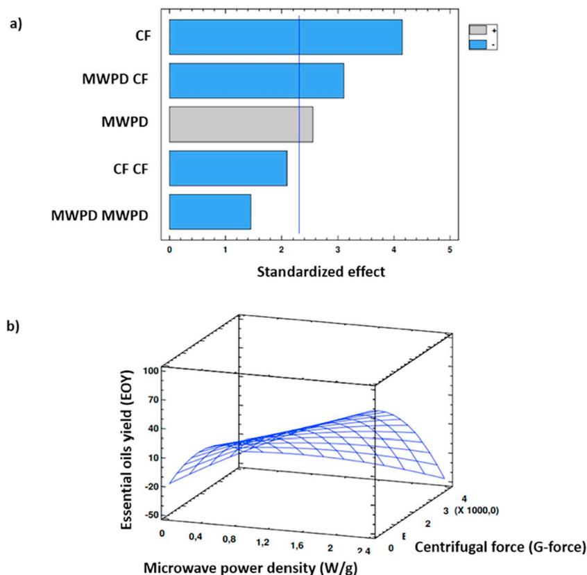
**Fig. 3.** a) Global yields standardized by Pareto chart with in blue color negative effect and gray color positive effect, and b) estimated response surface as a function of microwave power density (MWPD) and centrifugal force (CF).
