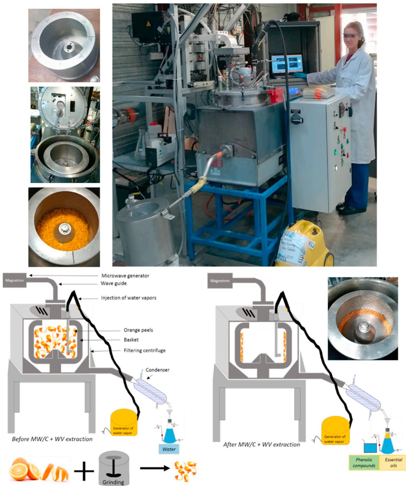
Fig. 2. Microwave-assisted dynamic extraction by combination with centrifugal force and water vapor before and after extraction.
